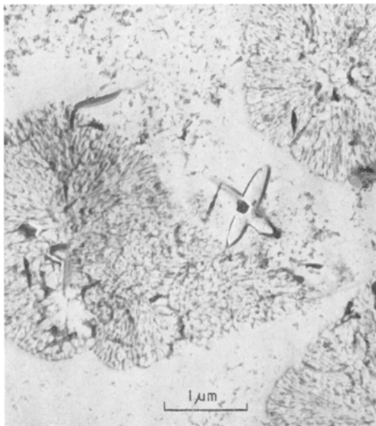
Figure 8 Secondary growth of twinned crystallites, presumably lithium titanate, following primary growth of the dendrites during \mu DTA of G69.
